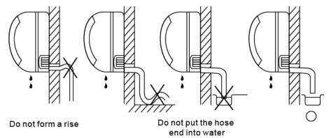
When connection extension drain hose, insulate the connecting part of extension drain hose with a shield pipe.
