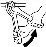
At the first debugging, completely expel air from coils via expelling valve.
