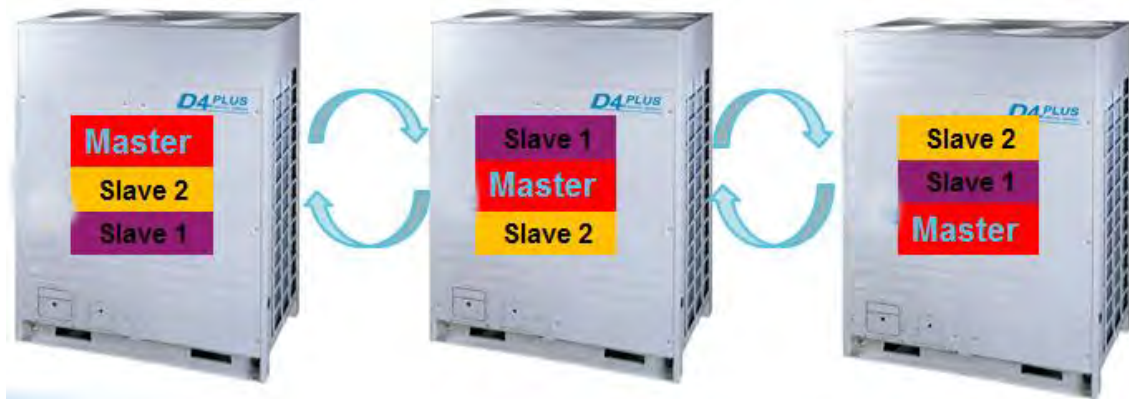
Cycle operation of outdoor units
