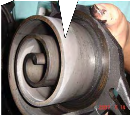
The bearing is worn seriously, it is damaged completely
