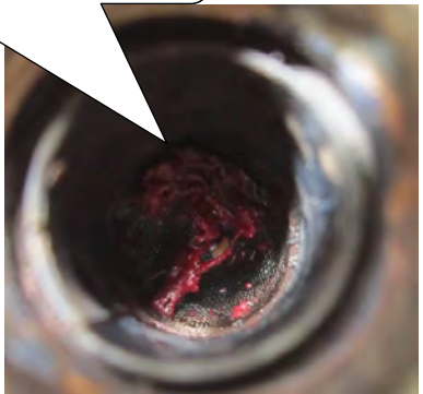
The filter is blocked by impurity, the suction of the compressor will be abnormal
