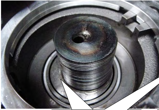
The crankshaft is worn.
