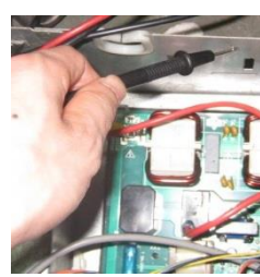
Figure 5-4.7: Measuring resistances between compressor terminals and ground
