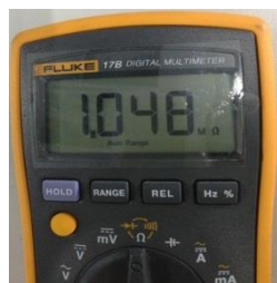
Figure 5-4.6: Measuring resistances among compressor terminals
