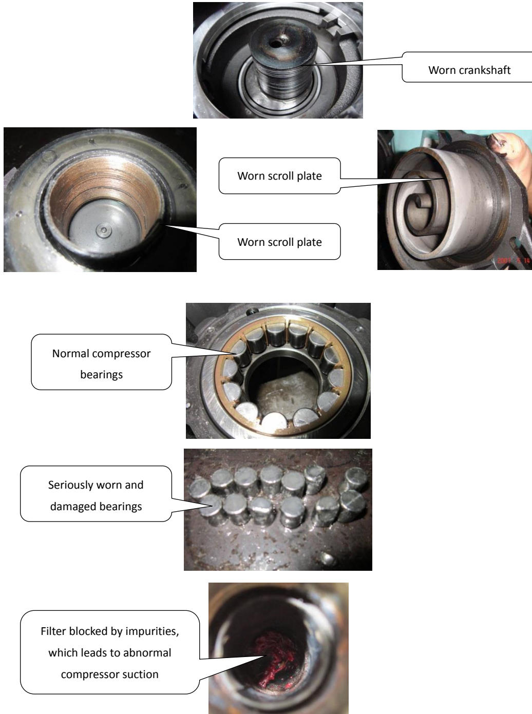
Figure 5-4.17: Effects of spoiled compressor oil
