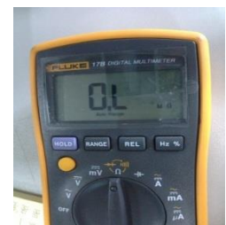
Figure 5-4.7: Measuring resistances between compressor terminals and ground
