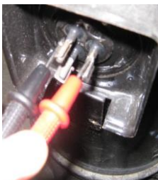
Figure 5-4.6: Measuring resistances among compressor terminals
